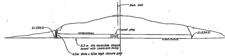
SECTION THROUGH DIVERSION TUNNEL
