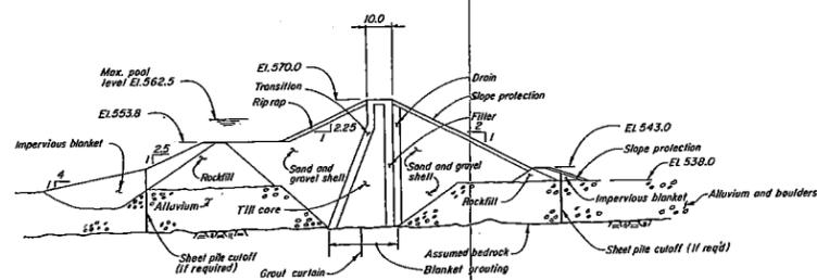
SECTION THROUGH EARTHFILL DAM
