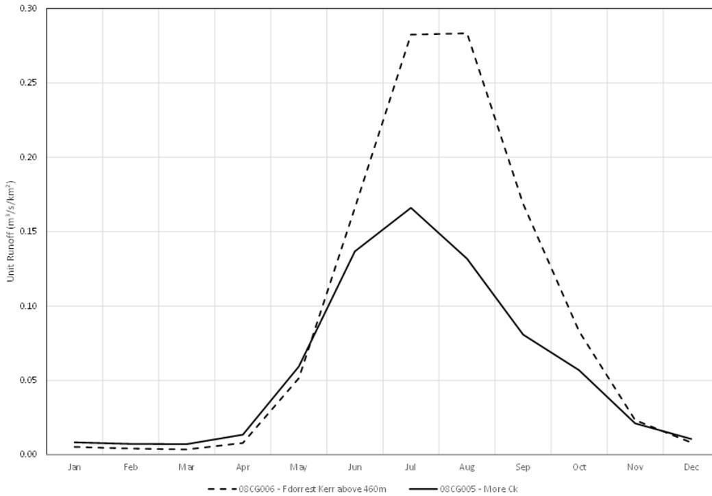
The average monthly flows at the project intake with and without the Forrest Kerr diversion are shown on Figure 2 below:
