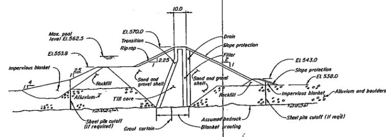
SECTION THROUGH EARTHFILL DAM
