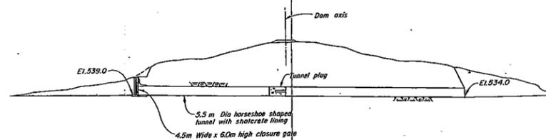
SECTION THROUGH DIVERSION TUNNEL
